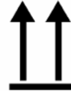
This way up The package must always be transported, handled and stored in such a way that the arrows always point upwards. Rolling, swinging, severe tipping or tumbling or other such handling must be avoided.
