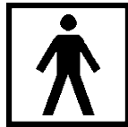
Type BF Applied Part (Marked beside the patient outputs)
